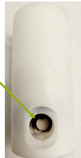
The separator will be moved up 3 mm to avoid stirring problems.
